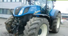
Bj. 2016, 3.950 h, 313 PS, AutoCommand Getriebe, 40 km/h, 220 l HighFlow Hydraulikpumpe, 5x DW, Fronthydr., Ber. v. 650/60 R34, h. 900/60 R42
